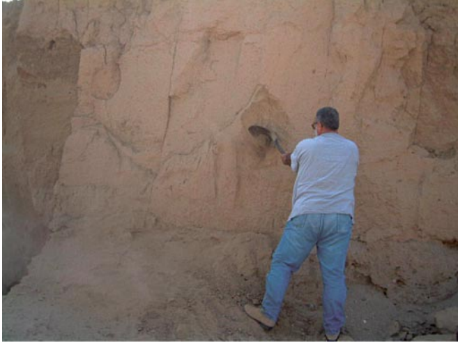
FIG. 2. Photograph showing vertical cliffs of loess deposits at old terraces in Al Sayl Al Kabir area, western region.
