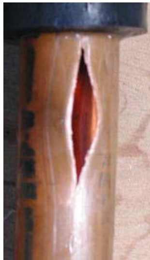
Fig. 7: The split formed at the central zone of the copper tube.
