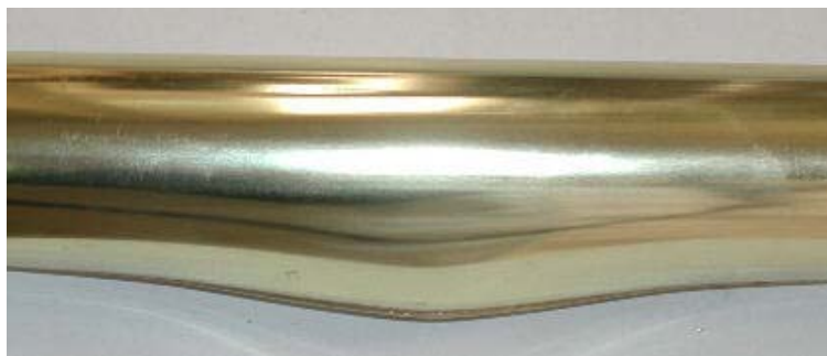
Fig. 13b: The bulging in the seam welded aluminum pipe.
